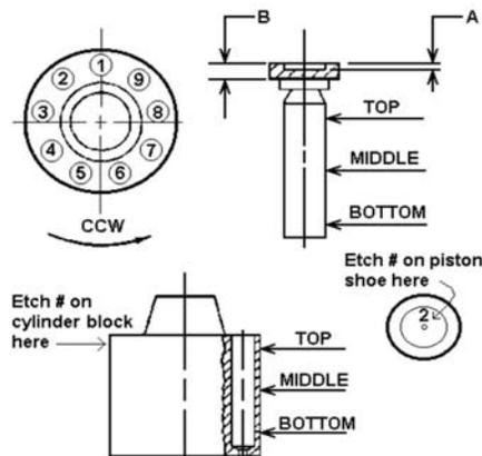
NOTE: In millimeters, measure cylinder barrel bores and piston OD to three decimal places (four decimal places if measuring in inches), and dimensions 'A' and 'B' to two decimal places (three decimal places if measuring in inches).
