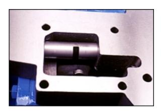
Carefully install the new remote electric control by aligning the fluid passage ports and retaining cap screws hole.
