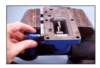
**Step 12**Using a 1/2 inch socket or open end wrench remove handle retaining nut, lock washer and handle from the shaft.
