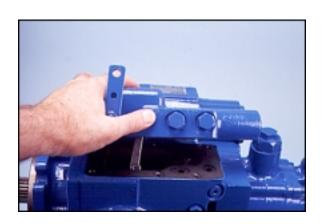
Remove the control gasket from the pump housing and discard.
