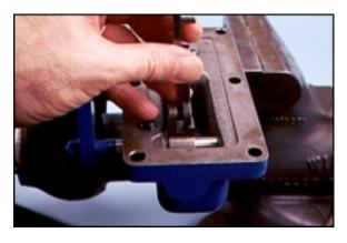
**Step 9**With the link assembly removed, remove the retaining ring and separate the two links.
