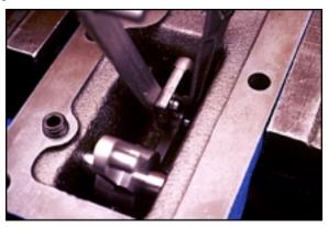
**Step 15**Center the shaft and align set screw with groove in the shaft.
