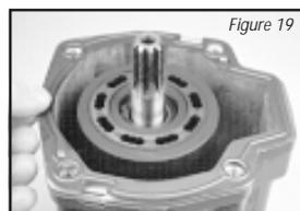
**21** Remove the valve plate from the piston block assembly. Note: This valve plate may have stuck to the endcover assembly that was previously removed.
