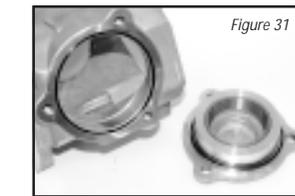
pump housing. Be sure to note on which side of the housing the control shaft protrudes before removing swashplate from housing for correct reassembly orientation.
