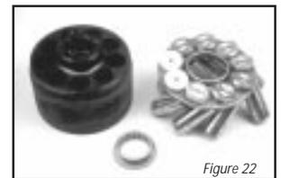
**25** Inspect the piston assemblies, spider, spider pivot and piston block. The piston block assembly usually requires no further disassembly unless the pins or block spring are damaged.
