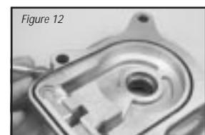
**12** Inspect the gerotor pocket and needle bearing located in the charge pump adapter. The needles in the needle bearing must remain intact in the bearing cage.
