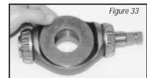
**37** Remove the thrust plate from the swashplate. The thrust plate is reversible and either side may face the swashplate (see Figure 33).
