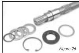
Note: The rear pump on tandem units uses a spacer in place of shaft seals.
