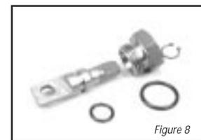
**8** Use a 1-1/8 in. socket or end wrench to remove the two high pressure relief valves from the pumps endcover assembly (see Figure 9). Remove plug, spring, and relief valve as shown from each side (see Figure 10). Each system relief valve assembly is identified by both its part number and relief valve setting as shown in Parts Information manual.
