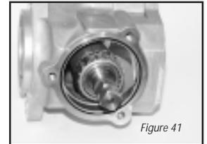
**10** Install the trunnion cover over the control shaft and into the pump housing. Install the three retaining cap screws and torque to 39,3 Nm [29 ft. lbs.] (see Figure 42).
