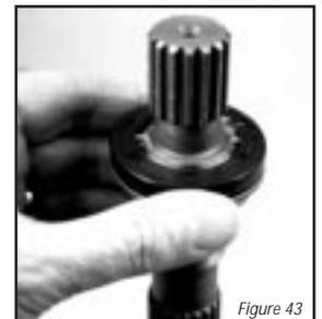
Note: The lip of the shaft seal must point toward the center of the input shaft.
