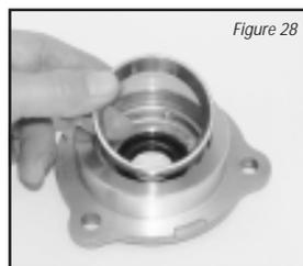
Note: The crush ring in the control arm trunnion cover does not need to be removed (see Figure 29). The only time the crush ring needs to be removed is when either the trunnion cover, the swashplate assembly or the housing assembly is replaced. A shim kit is then required in the crush rings place.
