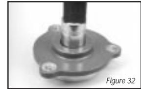
**36** To remove the control side cover plate lip seal, use a small press and press the lip seal inward (see Figure 32).
