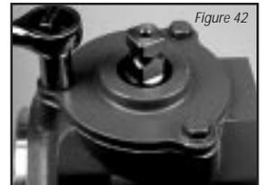
**11** Using your fingers, tilt the swashplate back and forth to check the trunnion bearing preload. Proper preload is achieved when the swashplate has a very slight tilting resistance. The swashplate must not have any or very little side clearance.
