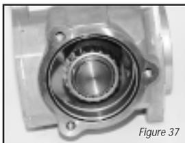
**4** Lubricate and install the o-ring seal into counter-bore of housing (see Figure 37).
