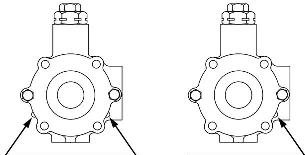
Clockwise rotation: bead on spacer and bead on pump body not aligned.
