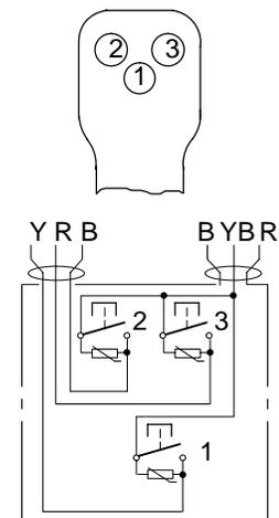
**Ergonomic Handle, Type X\*(P)\*: Switch and Wiring Configurations**
