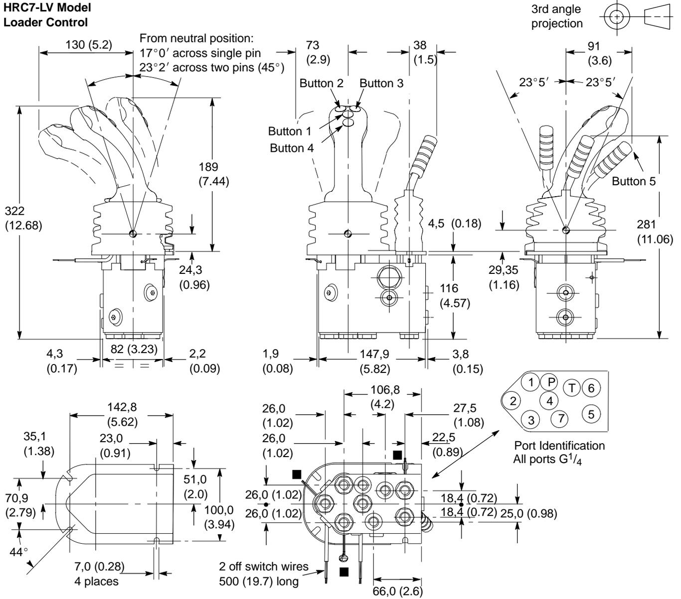
Detail of Flange Mounting Bolt Slots
