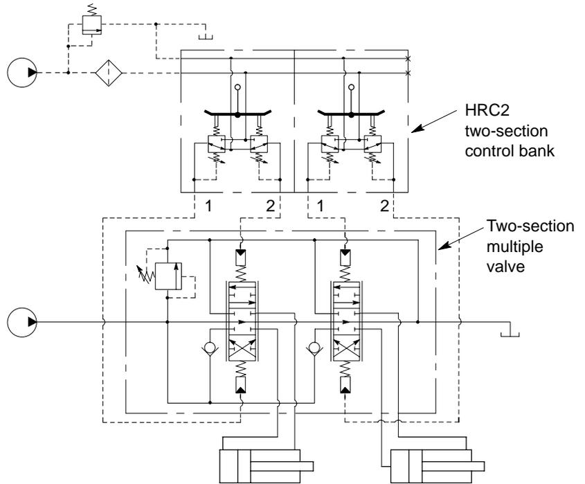
b. Stabilized input to HRC from an ACX2 accumulator unit. Two main pumps can be alternative sources for the ACX2/HRC pilot system.
