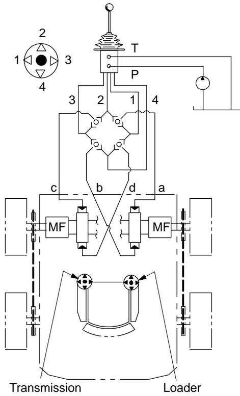
HRC4-TC applied to crawler with close-coupled hydraulic transmissions: variable-displacement pump and fixed-displacement motor.
