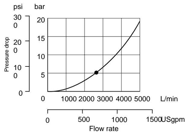
**Pressure Drop/Flow Through Insert
