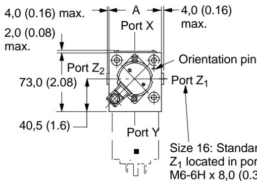
Size 16: Standard orifice Z<sub>1</sub> located in port Z<sub>1</sub>. M6-6H x 8,0 (0.3) deep
