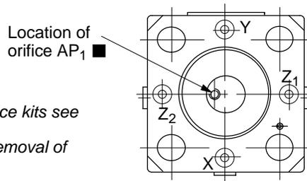
▲ Size 05 pilot control valve to be ordered separately. Typical model Vickers DG4V-5, see GB-C-2281.
