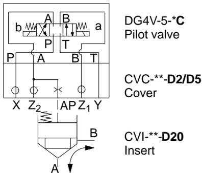
**Note that the circuitry (i.e. flow path and orifice locations) of these 50 and 63 sizes is different from that of sizes 16 to 40 shown on the previous page.**
