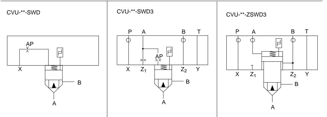
∧ Standard factory-fitted orifice.
