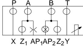
As can be modified for Normally Open function: interchange plug/orifice in AP<sub>1</sub>/AP<sub>2</sub>
