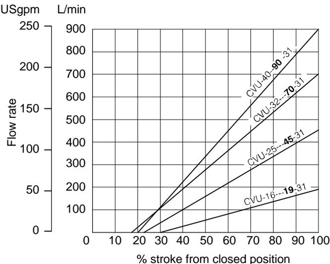
For a given input signal value the characteristics of the valve approximate to the theoretical square-law relationship for sharp-edged orifices:
