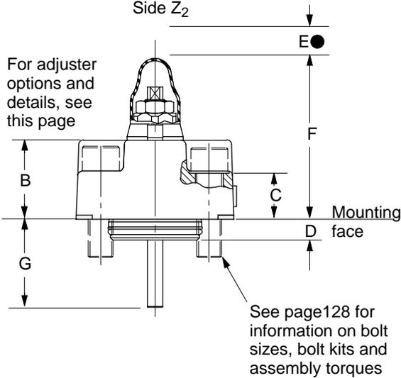
● Minimum clearance for removal of cover from manifold. For adjuster type K allow 43,0 (1.69) for key removal, see this page.
