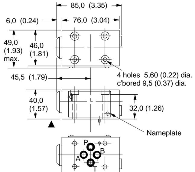
■ Mounting surface conforms to ISO 4401, size 03 (with additional orientation pin/pin hole); ANSI/B93.7M-D03.
