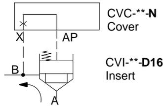
Used with the model D16 (1:1.6 area ratio poppet) insert, the combined cover and insert becomes a check valve. Port X in the cover is connected to port B in the insert. This allows free flow from insert port A to port B while blocking flow from B to A.
