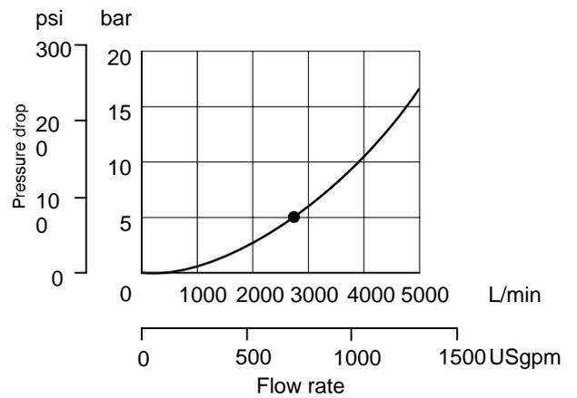
**Pressure Drop/Flow Through Insert
