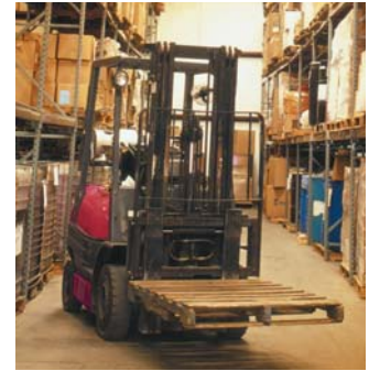
Lift truck with steer by wire
