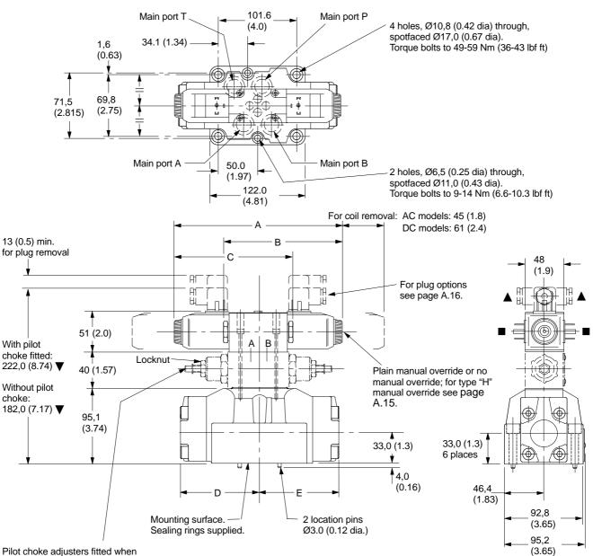
Pilot choke adjusters fitted when Model Code  $\boxed{4}$  = 2, 3, 27 or 28. To adjust, turn locknut counter-clockwise, then turn screw clockwise to slow down rate of spool travel, or counter-clockwise to increase the rate. Retighten locknut to 25-30 Nm (18-22 lbf ft).
