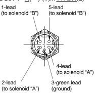
3-pin connector When fitted in single-solenoid valves, e.g.:
