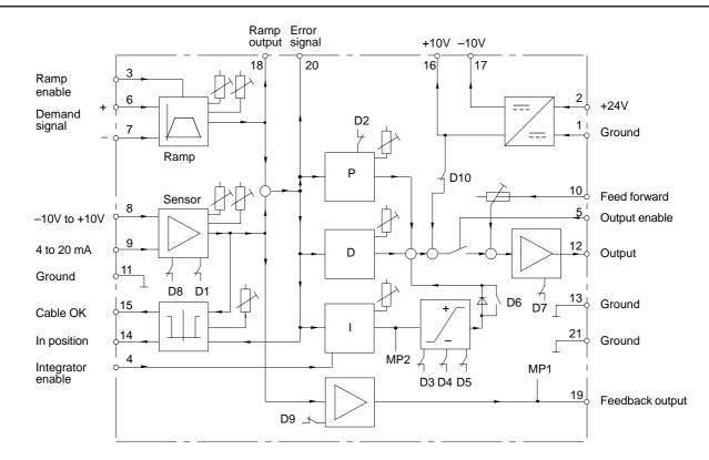
Note: The unused input signal pin 6 or 7 must be connected to signal OV (pin 11, 13 or 21).
