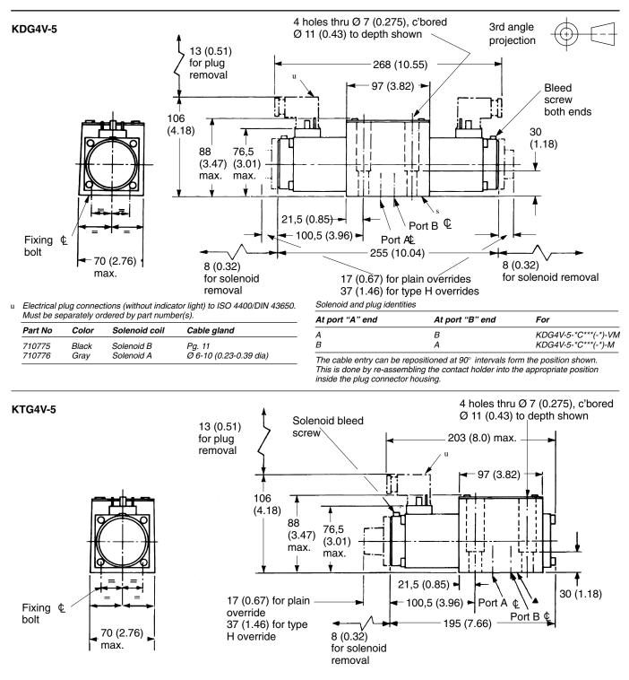
Electrical plug connections (without indicator light) to ISO 4400/DIN 43650. Must be separately ordered by part number(s).
