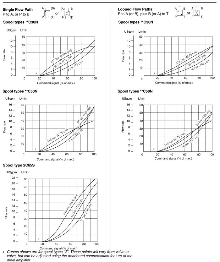
For spool types "33" the curves are similar but flow starts at slightly higher command signals.
