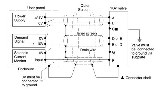
■ Solenoid current monitor voltage (pin F) will be referenced to the KA valve local ground. A "local ground" (pin C) is provided for optional use by differential input customer supplied electronics.
