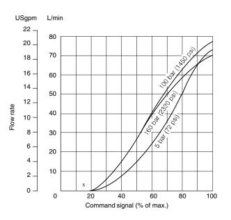
Maximum system pressures for this configuration: With "L" port externally drained .... 210 bar (3000 psi) With "L" port blocked ..... 160 bar (2320 psi)
