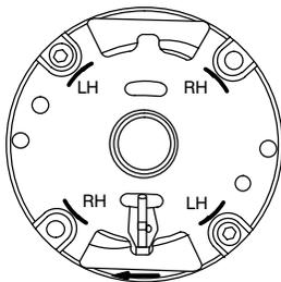
Sharp Edges of Vane Must Lead in Direction of Rotation
